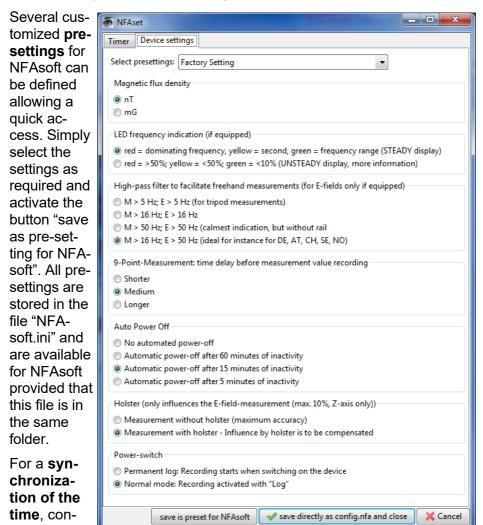
NFA (with SD card!) to the computer with the USB cable. Synchronization happens automatically, as soon as "CONFIG.NFA" is saved to the SD card. If a larger time lag persists, only a new SD card will help (see hint on page 10).
