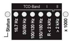
The **frequency-LEDs** change their colour ("traffic light principle").
